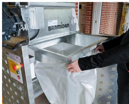
When the plastic bag is full with granulated material, you can easily exchange it with a new bag.
