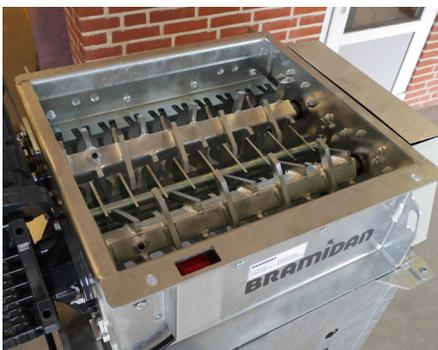
Polystyrene plates or boxes are efficiently granulated by the two-shaft rotors.
