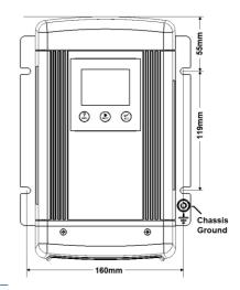
mark the positions of the fixing screws.
