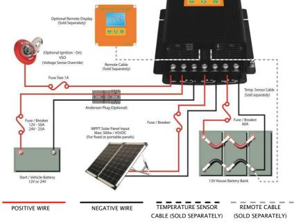
Note: This diagram is for a reference only. No cables, fuse/breakers, batteries or solar panels are supplied with this unit. Local rules and regulations should be followed when installing this unit.
