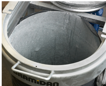
Compression inside a galvanized steel chamber prevents the bag from busting.
