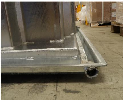
A draining system leads liquids out of your baler during compaction of wet waste.
