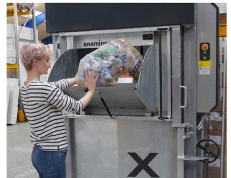
A flap door prevents back-run when filling PET bottles and cans into the chamber.
