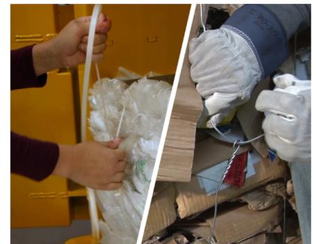
You can use either plastic strapping or baling wire to tie the finished bales.
