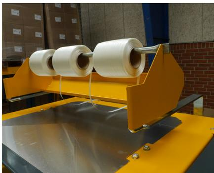
Strap holders on machine top eliminate going behind baler.
