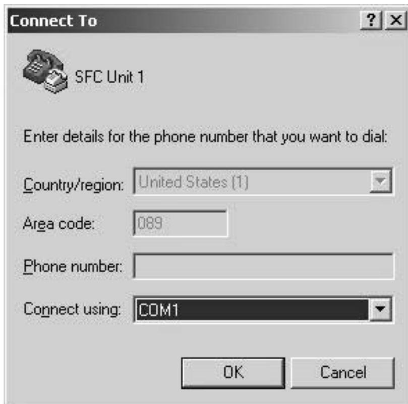
Select under "Connect using" the port to which you have connected the interface adapter, such as COM1.
