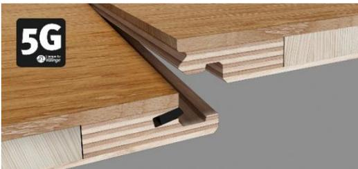
A distinct “click” sound signalling floorboards becoming locked together during installation. No extra tools needed for assembly. Optional locking of 2LOC boards (only on the long side of the board). Installation over an underfloor heating system is possible. Installation in the floating and glue-down systems.
