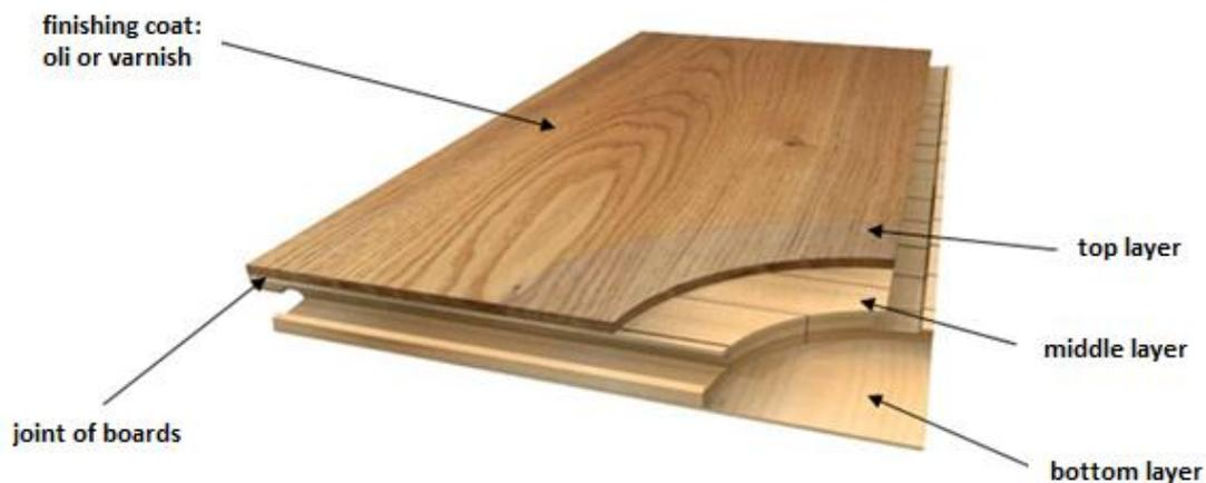
Fig. 2 Construction of a three-layer wooden floorboard offered by Moland A/S.
