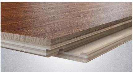
Floors with a total thickness of 14 mm and 21,3 mm, with a 3,5 mm-thick renovatable layer, which makes it possible to renovate the floor up to 3 times. They are installed in the 5G, T&G and 2LOC systems. The structure is made of spruce wood, which is characterized by high resistance to room humidity and temperature fluctuations throughout the year. The boards are finished with 7 coatings of varnish or 2 coatings of oil.
